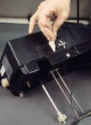
1.3 Stand the unit up so it is sitting on the rear of the Motor Unit and resting on the heating element.
