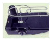
2.3 Put the new sealing tape (JOBO Part #70232) on the rotation motor side of the unit.
