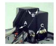
D. Lift off the rear cover to the upper head assembly.
