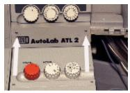
2) Pull the access panel forward being careful not to lose the rubber grommet(s) located on the right side of the panel.
