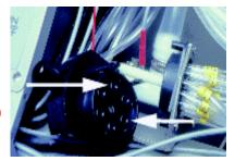
DO NOT remove the air hoses from the left half of the front/back bottle (air) switch!
