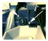
NOTE: There are a series of washers and O-rings or just an O-ring (depending upon the age and ATL model) located under the heads of the screws and/or behind the lift arm supports (the plastic piece behind the heads of the screws). Use caution when removing the screws so the O-rings will be become torn. Also use caution when removing the screws so you do not lose the O-rings or washers by dropping them into the bottom of the trough.
