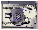
9) Observe the square hole in the center of the star-like gear with hose.
