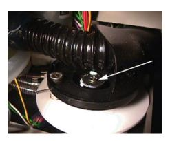
21) Loosen the #1 Phillips® screw a few turns. Then lift the large gear (located just below the drain arm) off of the small gear (located just below large gear and to the rear) to enable you to reposition the large gear so the drain arm is located over bottle #1's position on the reclamation device.
