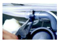
5) Disconnect the first four (4) air lines from the bottles, keeping the black plastic  $90^{\circ}$  angle elbows attached to the hoses.
