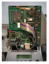
The largest cable is a round gray cable on which you will find a black locking connector. It is located toward the bottom of the electronics and enters the lower motor unit. Find the black locking connector and pull the cable apart at the connector.
