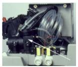
3) Locate the hose connected to the outlet of the air pump. The hose will be attached either by a wire tie (or Ty-wrap) or by silicon sealant. If the hose is attached with a wire tie, cut the wire tie and pull the hose off of the air pump. If the hose is attached with silicon sealant, simply pull the hose off of the air pump.
