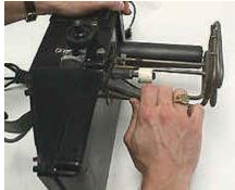
22.2. With the float switch unplugged from the circuit board, pull the defective float switch out from the bottom of the motor unit (lower head) using a downward "and to the side" movement.
