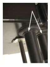
22.6. The O-ring should be barely visible from the bottom of the motor unit. The O-ring prevents the switch was rising up into the motor unit.
