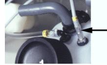
5. Disconnect all of the air lines from the bottles, keeping the black plastic  $90^{\circ}$  angle elbows attached to the hoses.
