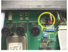
20.8.Remove the lower interface circuit board.
