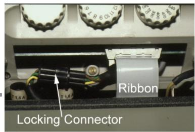
NOTE: This connection can be difficult to open! Do not use any tools to pry this connector apart!
