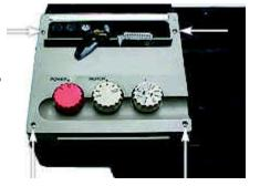
13. Located at the top of the ribbon cable, you will see a hinge or tab on both sides of the connector. Simultaneously move both hinges out and to the side and slightly upward. This action will push the ribbon cable connector downward out of its receptacle.
