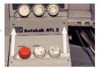
6) Pull the access panel forward being careful not to lose the rubber grommet(s) located on the right side of the panel.
