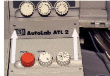
6) Pull the access panel forward being careful not to lose the rubber grommet(s) located on the right side of the panel.
