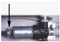
7) Disconnect the water bath heater electrical connection by prying down the metal locking clamp located at the bottom of the connector. Then unplug the connector by pulling out toward you.
