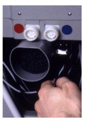
NOTE: After the wires are routed back through the lower motor unit, make sure you replace the sponge filter material back into the end of the wiring channel.
