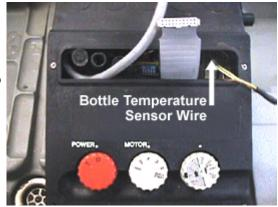
NOTE: The orientation of the connector for the bottle chemical temperature sensor is not important. As long as <u>all three pins male pins</u> are connected with the sensor, the sensor will function properly.
