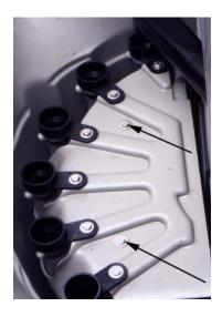
3. Push the chemical drain arm all the way back and lift up on the chemical reclamation plate just enough to prop it on the chemical drain arm. This will give you access to the bracket discussed in Part 11.
