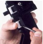
9.0 Insert the white retention clips. Make sure the bottom edge of the clips is underneath the black ledge molding located on the rear side of the lift arm. Use a small standard blade screwdriver to "encourage" the clip over the ledge molding.
