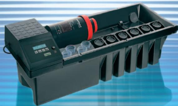
JOBBO CPP-3 # 4083 for magnetic rotation of developing tanks. Coupling on and off of tanks for changing solutions with running motor. JOBO inversion tanks must be equipped with magnet # 1504 and for use with Lift with cog # 1505. Not acceptable for Expert Drums.
