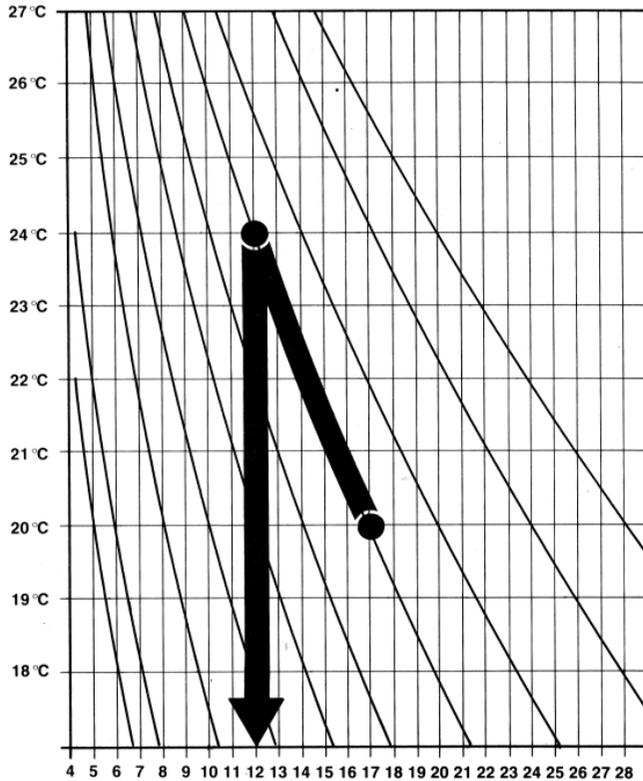
The maximum allowable temperature difference is +4°C from the selected process temperature. If the difference is higher, the process will stop displaying: "out of range". Take 24°C-processes in-stead of 20°-processes, if 20°C-process is out of range.
