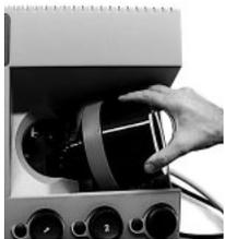
Mount the tank to the processor.
