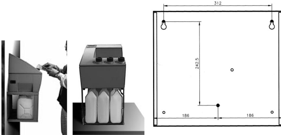
The processor should be positioned with the feet in location holes in the reclamation unit. The drain outlets for the three chemistry baths locate in the storage containers without the need of interconnecting hoses. Drain hoses for rinse water and water jacket must be connected. When lowering the processor, take care that the outlets adapt to the tubes of the reclamation rack.
