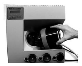
Press the START button. The tank will rotate during a 5 to 7 minute pre-warm cycle, and then the process will start automatically.
