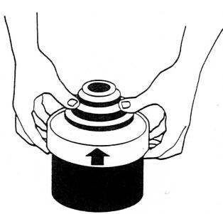
Check that the stopper used for print processing (#15042) is removed from the funnel.
