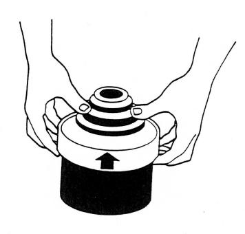
Place stopper (Part #15042) into the funnel to prevent light leaks. (The center core is not used when processing prints.)
