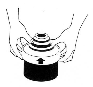
Adjust the reel to the proper film size  $(4x5^n, 6x9 \text{ cm or } 9x12 \text{ cm})$  by holding one half in each hand and rotating the left spiral clockwise until it can be slid to the proper width for the film to be loaded.
