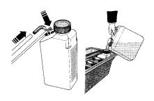
Firmly screw on bottle lid, press air hose and elbow and push solution feed hose onto rising pipe(37).
