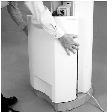
When fitting the front panel, ensure that the 3 nipples at the top and the 2 open elongated holes at the bottom engage in the yellow pins. Then tighten the screw on the front side, using the flat screwdriver.
