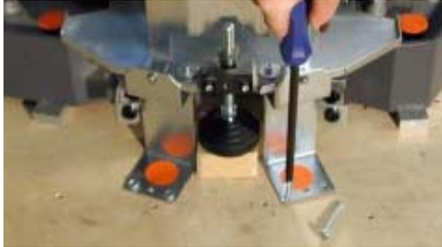
Remove the 2 wood screws from the pallet for each of the two transport brackets. You will require the Phillips screwdriver for this. Subsequently loosen the brackets from the magazine table mounting posts, using a flat screwdriver.
