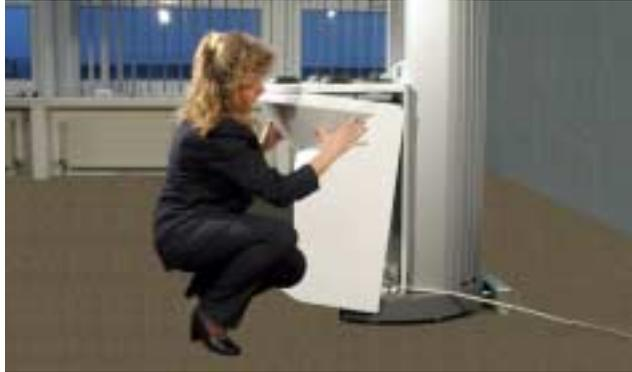
Tilt the top of the front panel towards the unit. Then guide the top edge of the front panel into the groove in the unit, until it fits the unit. Subsequently press the bottom of the panel towards the unit and screw it down using the flat screwdriver.
