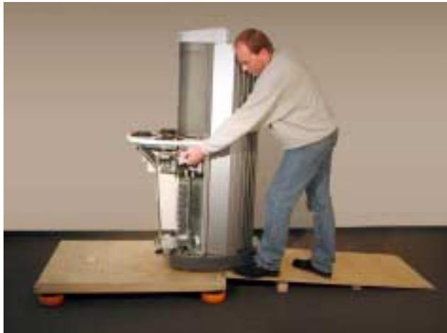
Do this by taking hold of the cast iron mounting and not parts of the magazine table.
