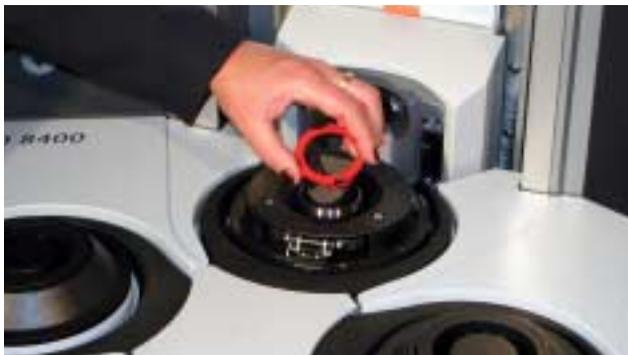
Carefully remove the transport safeguard, which is clamped onto the transparency arm.
