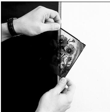
Hold transparency originals against a dark background and then in front of and against a light background. Observe the original from different angles and distances. Determine whether it is soiled or not and if so, the type of soiling.
