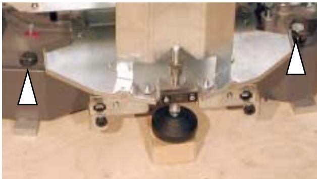
Remove the two wood screws attached to the base, using the 17 mm open-ended wrench.
