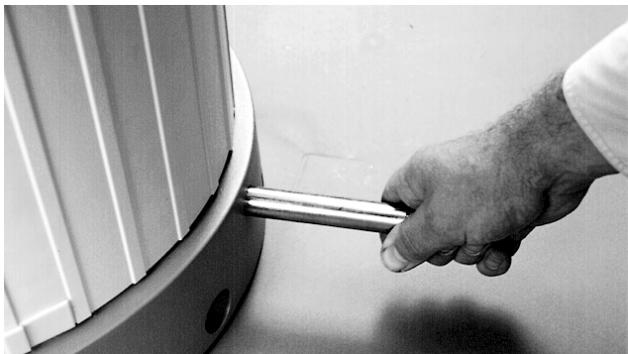
Pull the transport safeguard bar out from the rear of the unit.
