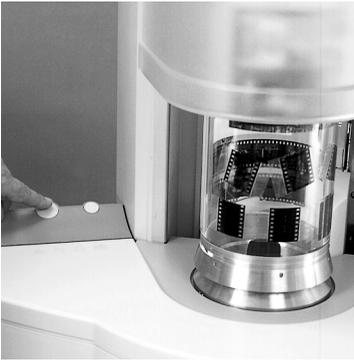
The drum change key is used to open the cover and release the drum for changing. Once the drum has been changed, the cover is closed again by pressing the key and the drum is locked. The unit is ready for scanning.
