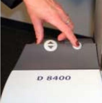
Operate the ON/OFF switch on the unit.
