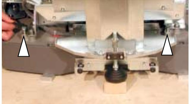
Screw in the two screws on the front side of the scanner up to the limit, using the 13 mm open-ended wrench.
