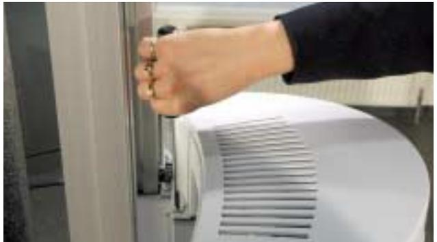
Fit the cover and secure it, using the M 6x6 screws from the accessories box.
