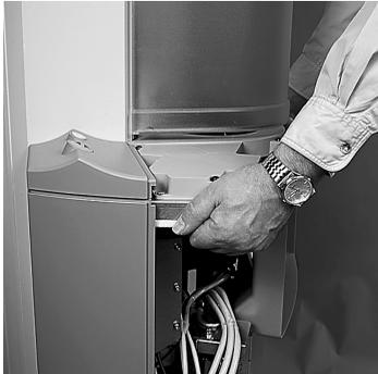
To negotiate bends, you can rotate the scanner to the right direction by raising the carrying plate on one side.
