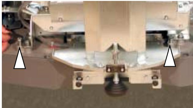
The rollers must be retracted once the scanner has been brought to its intended final location. To do this, turn back the screws until they rotate freely. You will need the 13 mm open-ended wrench for this.
