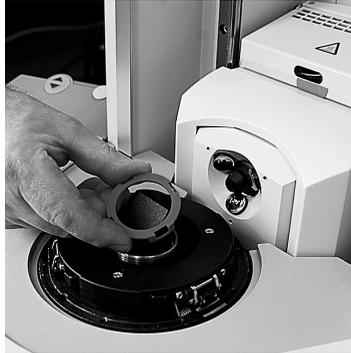
Carefully remove the transport safeguard, which is clamped onto the transparency arm.
