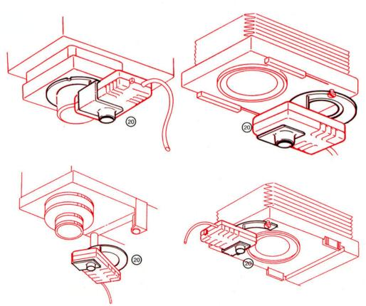
The Jobotronic 2000 quartz is a digital automatic timer and enlarging exposure meter with quartz-stabilised time control and highly sensitive silicon meter probe.
