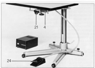
The baseboard is adjusted by means of a servo mechanism. To do this, slacken off the large locking knob (21) at the front right of the baseboard arm (4), grip the baseboard slightly behind the centre by the two lateral edges and press the pedal (24). The baseboard can then be raised or lowered without effort.
