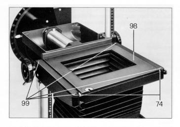
The supporting plate (98) for the negative carrier must also be changed. Unscrew the four screws, remove the old supporting plate and fix the new supporting plate with the four new screws (99). The bearing rollers (74) should be at the front of the negative carrier holder.
