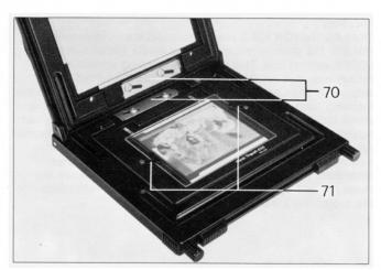
When using the TRIGRAFI 66 or 450 register inserts, remove both glasses from the TRINEG carrier after first pushing aside the catches (70) at the rear ends of the TRINEG. Insert the TRIGRAFI register insert required in the lower section of the negative carrier and secure with the sliding catch (70). The film placed on the lower glass plate of the TRIGRAFI register insert is pressed down by the upper glass plate and the springs (71).
