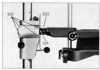
The following further step is required before mounting the new CLS 1000 colour head on the LABORATOR 138 S: Move the carrying arm (100) complete with the enlarger head forward by about 4.5 cm. This can easily be done slackening the four socket head bolts (103). Also unscrew the scale pointer mounted on the enlarger head and replace it with the new scale pointer (101) supplied in the kit.
