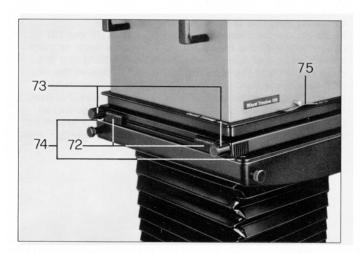
The TRINEG negative carrier has individually adjustable masking strips to mask down the image area. Use the two sliding controls (72) on the negative carrier for horizontal mask adjustment and the knobs (73) for vertical adjustment. Do not use the masking strips as format masks.
